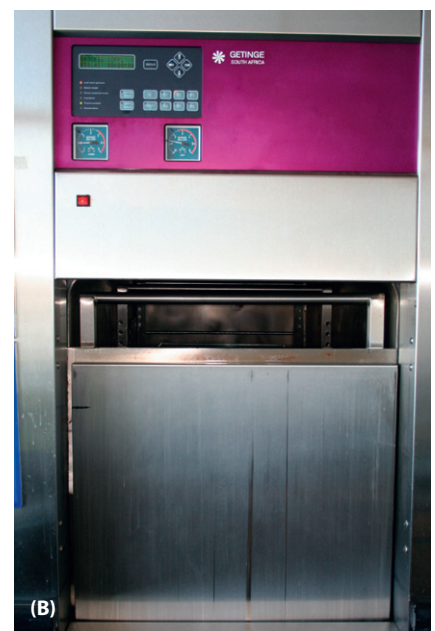
Fig. 3 (A) Top-loading and (B) front-loading autoclaves. Different sizes are used, depending on the needs of the facility.
